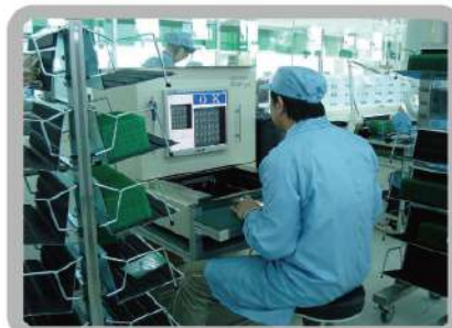
OMRON RNS-pt AOI tabletop inspection system
