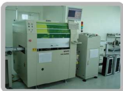
MINAMI Fully automatic in-line printer & Loader DER-2535L
